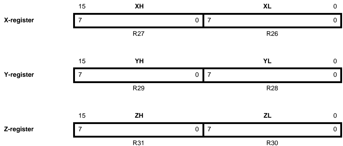
Figure 4-3. The X-, Y-, and Z-registers
